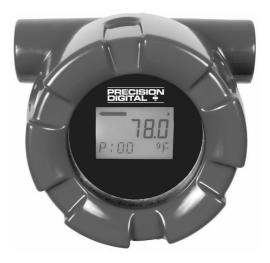
The instrument enclosure is a cylindrical single compartment enclosure comprising a base and cover with a maximum internal volume of up to 298cm<sup>3</sup>, and may be manufactured from cast aluminium or stainless steel depending on enclosure type, which may include an epoxy paint finish.
