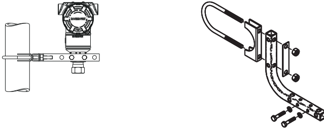
Figure 3-6: Pipe Mount Rosemount 3051T
