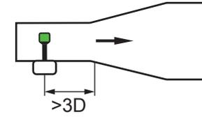
Place the sensor in front of the diffusers at a position with high air velocity.
