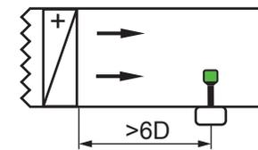
Place the sensor at a position with laminar (non turbulent) flow. Turbulence appear after fans as well as after bends, junctions, air heater, air cooler, filters, flaps or diameter changes in the duct.
