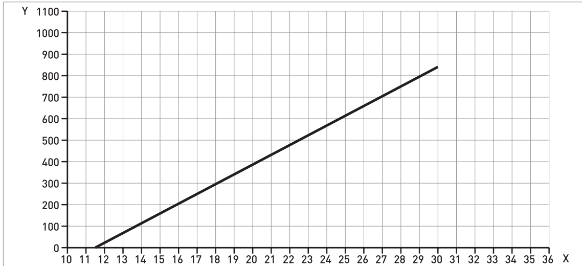
Figure 2-1: Minimum power supply voltage for an output of 22 mA at the terminal (Non-Ex and Hazardous Location approval (Ex i / IS))
