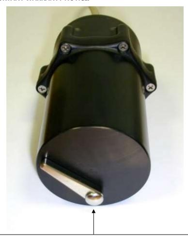
THE ONE YEAR TRANSDUCER WARRANTY IS VOID IF THE WIPER BLADE IS ROTATED BY HAND. THIS IS DETRIMENTAL TO THE MOTOR GEAR DRIVE AND WILL DAMAGE THE UNIT.
