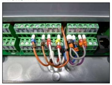
The transmitter unit has two analogue outputs and two digital outputs. Channel 1 is mA OUT 1. Channel 2 is mA OUT 2.
