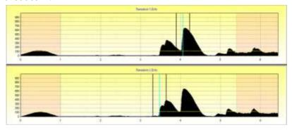
The above profiles show the unit differentiating between the two echoes. In this instance point one is set to pick the largest echo and point two is set to pick the first echo (see SF2 Service Manual for details).
