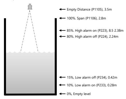
In this example, when the level rises to 2.38 m, relay 2 will come on until the level drops to 2.24 m when it will turn off. If the level drops to 0.28 m, then relay 3 will come on until it rises 0.42 m when it will turn off.
