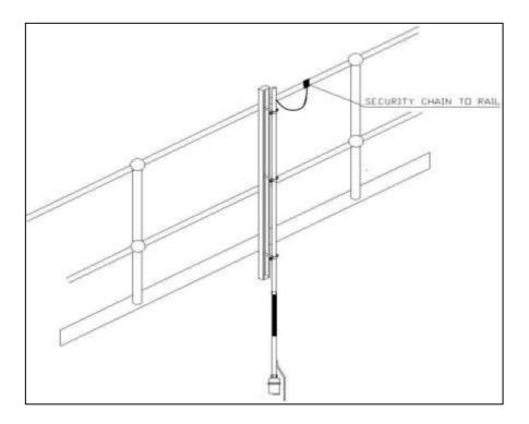
This mounting system has galvanised parts and is designed to be a budget option for transducer mounting.
