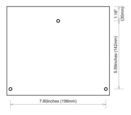
The Sludge Finder 2 should be mounted by drilling three holes suitable for size 8 screws (length to suit your application) and fixing the top screw in place. Hang the unit on this and fix the two remaining screws by removing the terminals access cover to access the pre-drilled holes.
