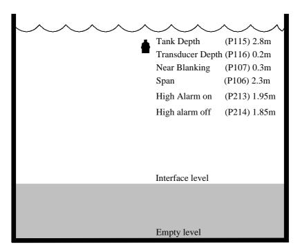
In this example, when the sludge interface level rises to 1.95 m, relay 1 will come on until the level drops to 1.85 m when it will turn off.
