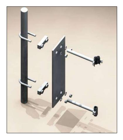
**Note:** the two arms holding the hinged conduit retainers are welded to the mounting plate.
