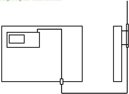
The Integrator on the Bridge should be protected from the elements inside an enclosure, the Antenna extension cable should be installed through a cable gland in the base of the enclosure and out to a suitable position so that the Antenna is above the enclosure.
