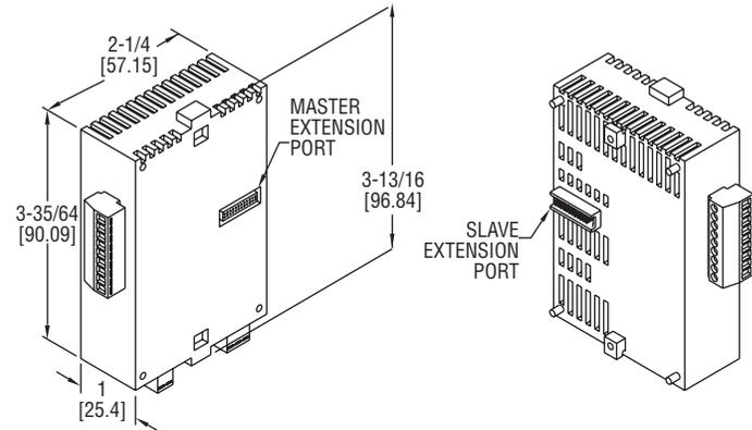
The DIN Rail Mount **SERIES SCD** offers multiple PID loops in a compact size. Each SCD-1000 master controller can be combined with up to seven SCD-2000 slave controllers without any wires. Each controller has one universal input, one relay output and one user selected output.
