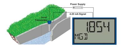
The PD4-6624, in combination with an ultrasonic level transmitter, makes for an economical way to measure and display open channel flow rate and total in most weirs and flumes. A guide such as the ISCO Open Channel Flow Measurement Handbook can provide the user with all the information needed: the exponent used in the flow equation for the desired flow units and the flow rate for any given head height.
