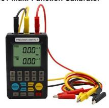
This <u>PD9501</u> Multi-Function Calibrator has a variety of signal measurement and output functions, including voltage, current, thermocouple, and RTD.
