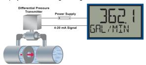
PD4-6624 Displaying Flow Rate by Applying the Square Root Function to the Output of a DP Transmitter.
