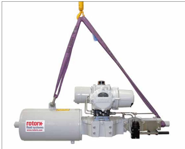
Fig. 4.1.1. SI3 lifting: Slings attached to the lifting eye and hydraulic cylinder stop bolt cover.
