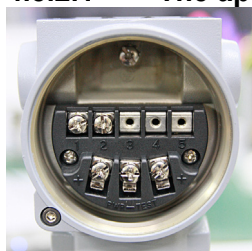
1 : Pulse Output+ , 2 : Pulse Output-
