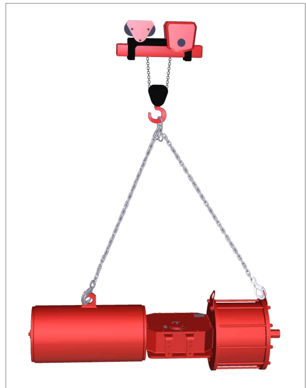
Fig 7.1 Lifting (single-acting actuator up to size 161)
