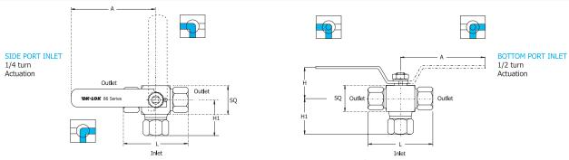
V86 3-way ball valve is designed to switch media through the inlet port and direct it to out of two outlet ports.
