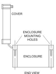
Note: This non-metallic enclosure does not automatically provide grounding between conduit connections. Grounding must be provided as part of the installation. Ground in accordance with the requirements of the National Electrical Code. System grounding is provided by connecting grounding wires from all conduit entries to the steel mounting plate or another point which provides continuity.
