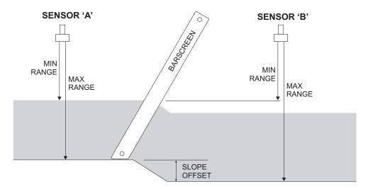
Slope Offst Appears when calibrating Sensor B. Enter a slope offset value to compensate for a sloped channel floor. Offset will be a positive value when Sensor B channel floor is lower than Sensor A channel floor.
