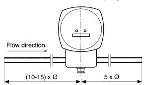
In order to obtain a fully developed flow profile through the instrument, the pipe run should be straight and should not contain any elbows bends or fittings. A free pipe run of 10-15 times the pipe bore upstream and 5 times downstream of the meter is recommended. Hose connection with area reducing hose nipples, if desired, should be installed only after this run.
