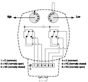
measuring range into 5 equal parts. If it is desired to have a switchpoint at 50% of maximum flow the switch adjusting dial would be adjusted to 2.5, etc. An adjusting tool is included with the unit and is clipped inside the cover. Adjust the switchpoint with the adjusting tool.
