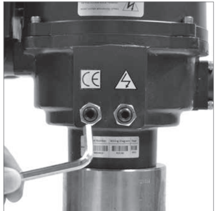
Setting anti-clock to close stop bolt
