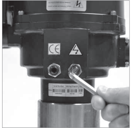
Setting clockwise to close stop bolt
