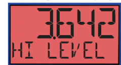
Meter in alarm condition. Display turns red, flashes and shows HI LEVEL alarm message.
