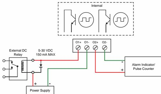
Figure 15. Open Collector Output Connections
