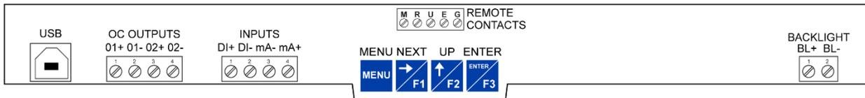
Figure 8. Connector Labeling for PD4-66XX-LNN
