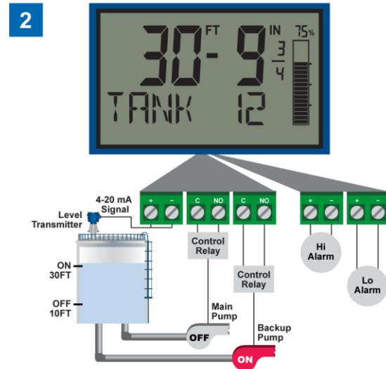
With the Pump Alternation feature activated, the next time the level reaches 30 feet, relay #1 transfers and starts the backup pump.
