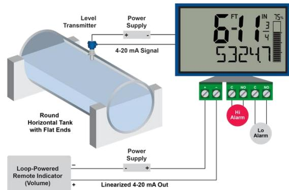
**PD4-6603 or PD4-6607 Displaying Height in Feet & Inches on Top Display and Volume in Gallons on the Bottom Display using the RHT Linearization Function.**
