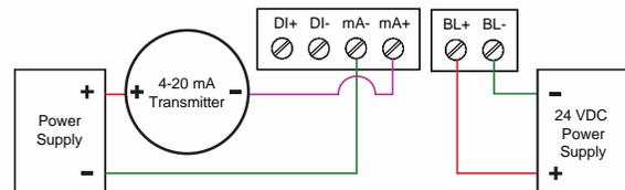
Figure 11. 4-20 mA Input Connection with Backlight
