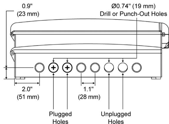
Figure 5. Conduit Holes Location - Bottom View
