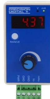
The [PD9502](#) is a low-cost, compact, simple to use 4-20 mA or 0-10 VDC signal generator. It can easily be set for 0-20 mA, 4-20 mA, 0-10 V or 2-10 V ranges. Signal adjustment is made with a one-turn knob. A wall plug is provided with the instrument. Optional USB power bank is available.
