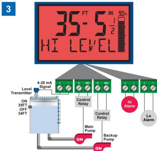
If the backup pump is not able to keep up, and the level reaches 35 feet, relay #2 transfers and starts the main pump as well. Open collector #1 trips the High Level Alarm, the display turns red and flashes "Hi Level" message indicating an alarm condition. The High Level Alarm resets at 34 feet.
