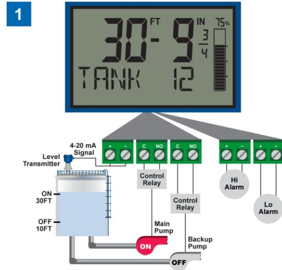
Relay #2 turns the main pump on at 30 feet and turns it off at 10 feet.
