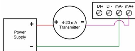
Figure 10. 4-20 mA Input Connection without Backlight
