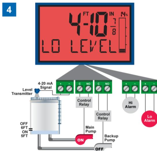
Once the level has dropped below the reset points, both relays will turn off. If the Main Pump fails to turn off, open collector #2 trips the Low Level Alarm at 5 feet to warn against the pump running dry. The Low Level Alarm resets at 6 feet.
